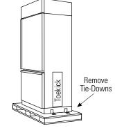
• Remove the four 7/16" bolts securing the straps to the skid.
